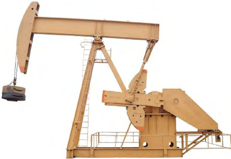
Crank balanced Pumping units
